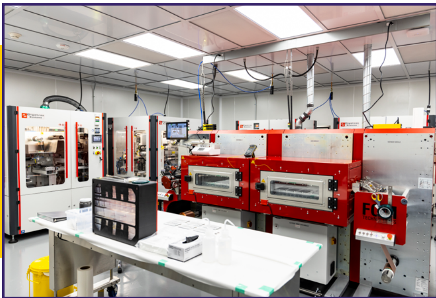
The dry room in the new battery lab at the Washington Clean Energy Testbeds features an FOM Technologies roll-to-roll coater for battery electrodes, and Digatron equipment for each step of the pouch cell assembly process. (Dennis Wise / UW Photo)
