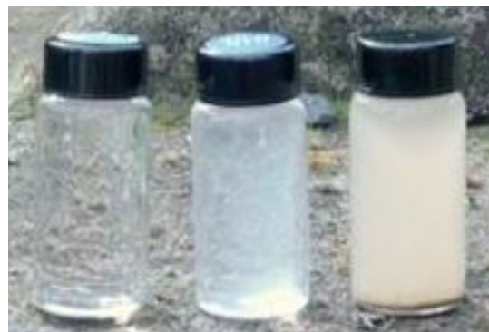
Light scattering from particles (e.g. lake sediment)
