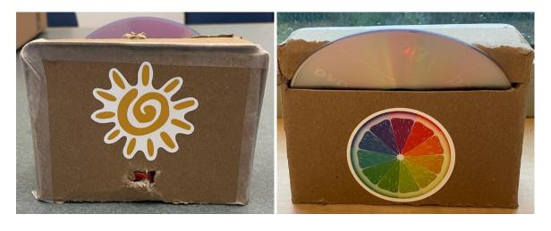
**STEP 5** Hold the spectroscope up to the sun and look through the viewing port.
