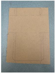
**STEP 2**Using scissors or an X-Acto knife, cut the cardboard along the black lines.
