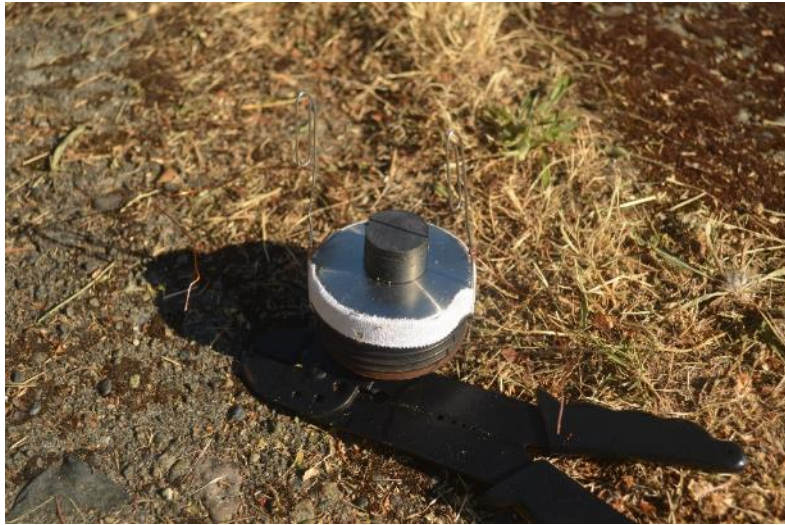
Neodymium magnet placed on the base of the motor.
