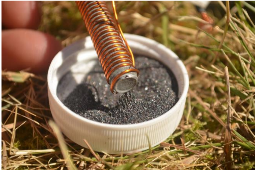
Electromagnet attracting iron fillings
