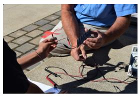
from .5 to 1.5 volts, each cell within the panel contributes .5 volts
