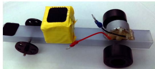
Wires connected to motor lugs
