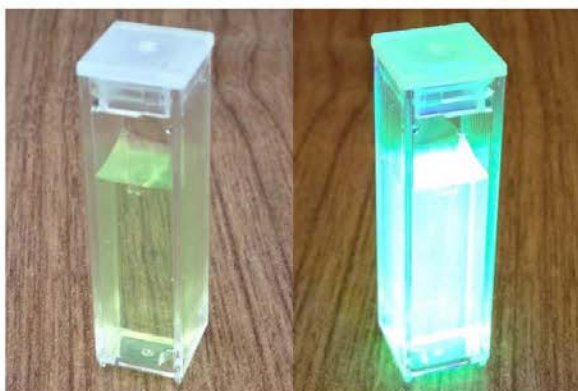
Ground state (no emission) Fluorescence (emission due to excitation)
