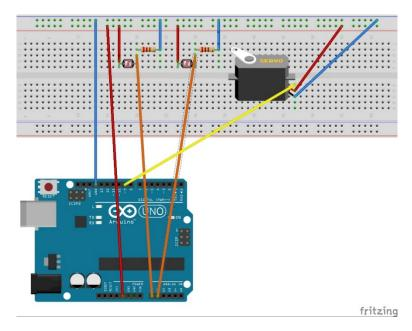
3. If you are doing this as a class this would be a time to brainstorm a pseudo-code description of what the program needs to do. Basically if L > R then turn the servo one way, else rotate the other. You need a tolerance factor for the minimum difference so that it doesn't just jitter with fluctuating measurements from the sensors.
