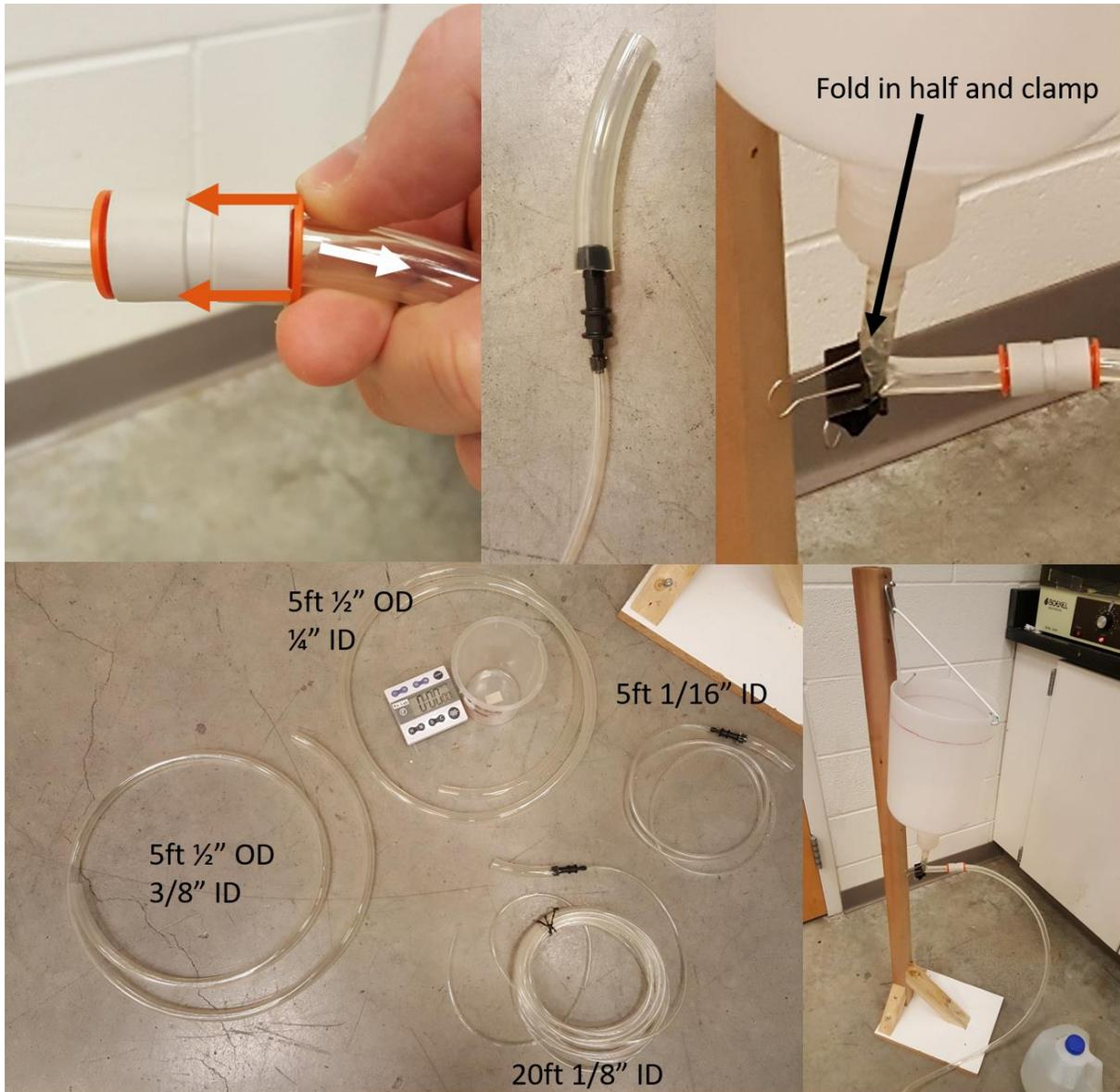
Cut a short length, around 4" of the 3/8" ID tube, and push it over the threaded barbed adapter. For the push-to-connect adapter, push it over the other end of the 3/8" ID tube as deep as it will go. Give it a gentle tug to make sure it's secure. To disconnect, pull the tube gently away from the connector while pushing inwards on the orange disk.
