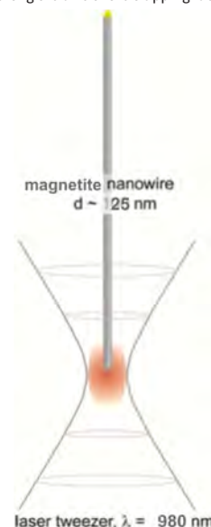
Figure 7: Nanowire oriented along the axis of the trapping laser, with a profile of laser intensity.
