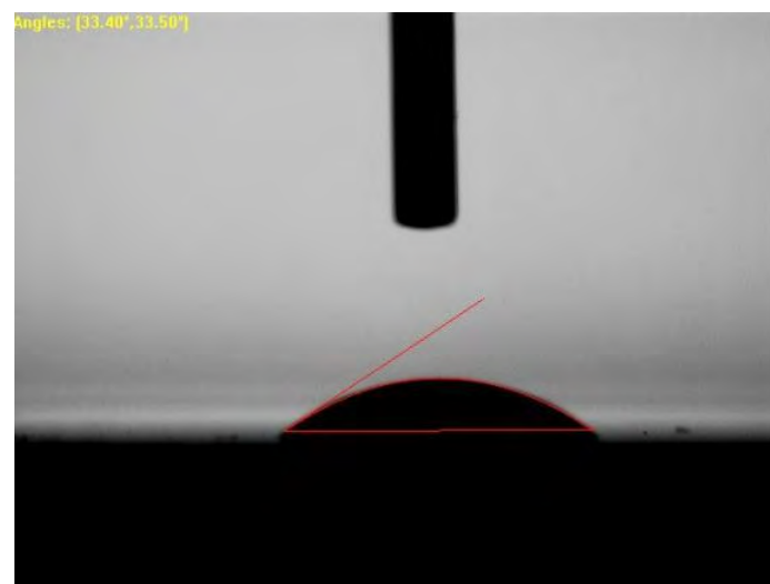
Figure 8: Contact angle measurement of clean SiO 2 substrate (first set).
