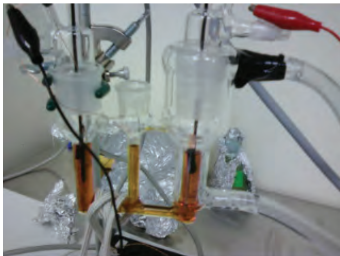
Figure 2. Shows the galvanic thermocell set-up.
