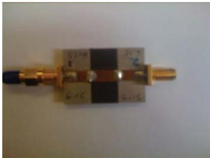
Fig. 4. Physical REMS model, three-segment microstrip.
