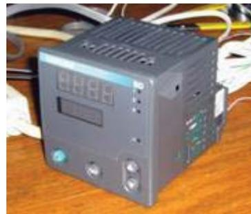
Fig. 2. Watlow temperature controller. In normal operation, upper display shows actual temperature and lower display shows set temperature.
