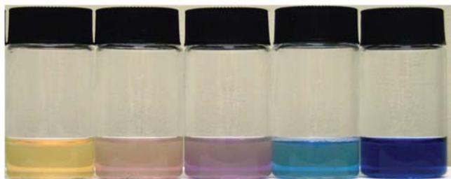
Figure 4. Photo of assorted thermal nanoprism colloids arranged in order of increasing borohydride concentration.
