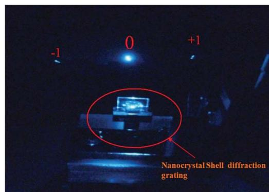
Figure 8: An argon laser (1.5mW) at an angle of 33.5°, showing the diffraction of the core/shell diffraction grating.
