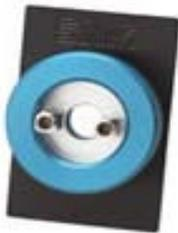
Figure 9. Demountable liquid cell used to assemble dielectric and metallic Fabry-Perot cavities.
