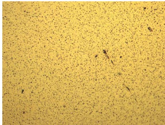
Figure 1. Microscope image of a calcium sample encapsulated with two-part epoxy after being exposed to 20°C and 50% RH for a week.
