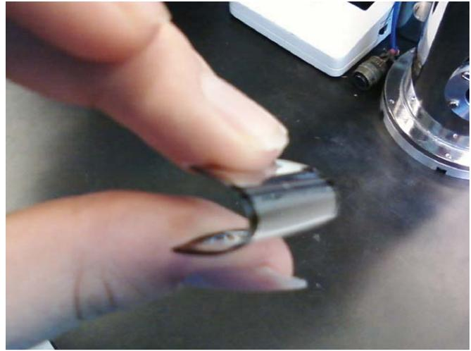
Figure 7. Image of two flexible plastic substrates sealed with a Poly-isobutylene sealant demonstrates the flexibility of this encapsulation method.
