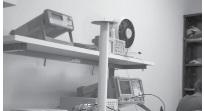
FIGURE 1A: Receiver apparatus, mounted to a linear positioner.
