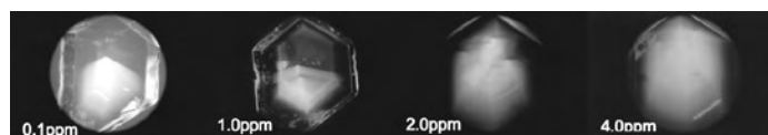
FIGURE 6. As \text{Ce}^{3+} concentration increases (from left to right), the boundary between the fast and slow slope increases progressively until dye enters the entire (010) face.
