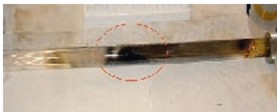
Figure 3. The “hot zone” is circled in red in figure 3 and indicated by the blackened nanotubes area.
