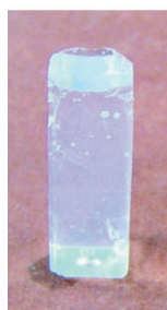
Figure 6. a) Fluorescence spectrum of a CdSe loaded sol-gel monolith, b) A picture of a sol-gel containing nanoparticles.
