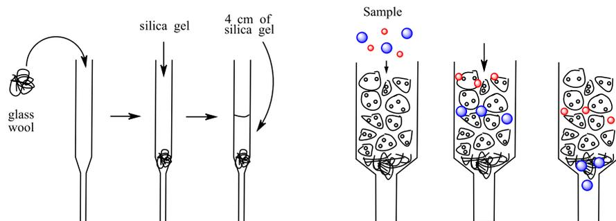
Figure 2. a) Building a silica gel column. b) The size-exclusion separation process.
