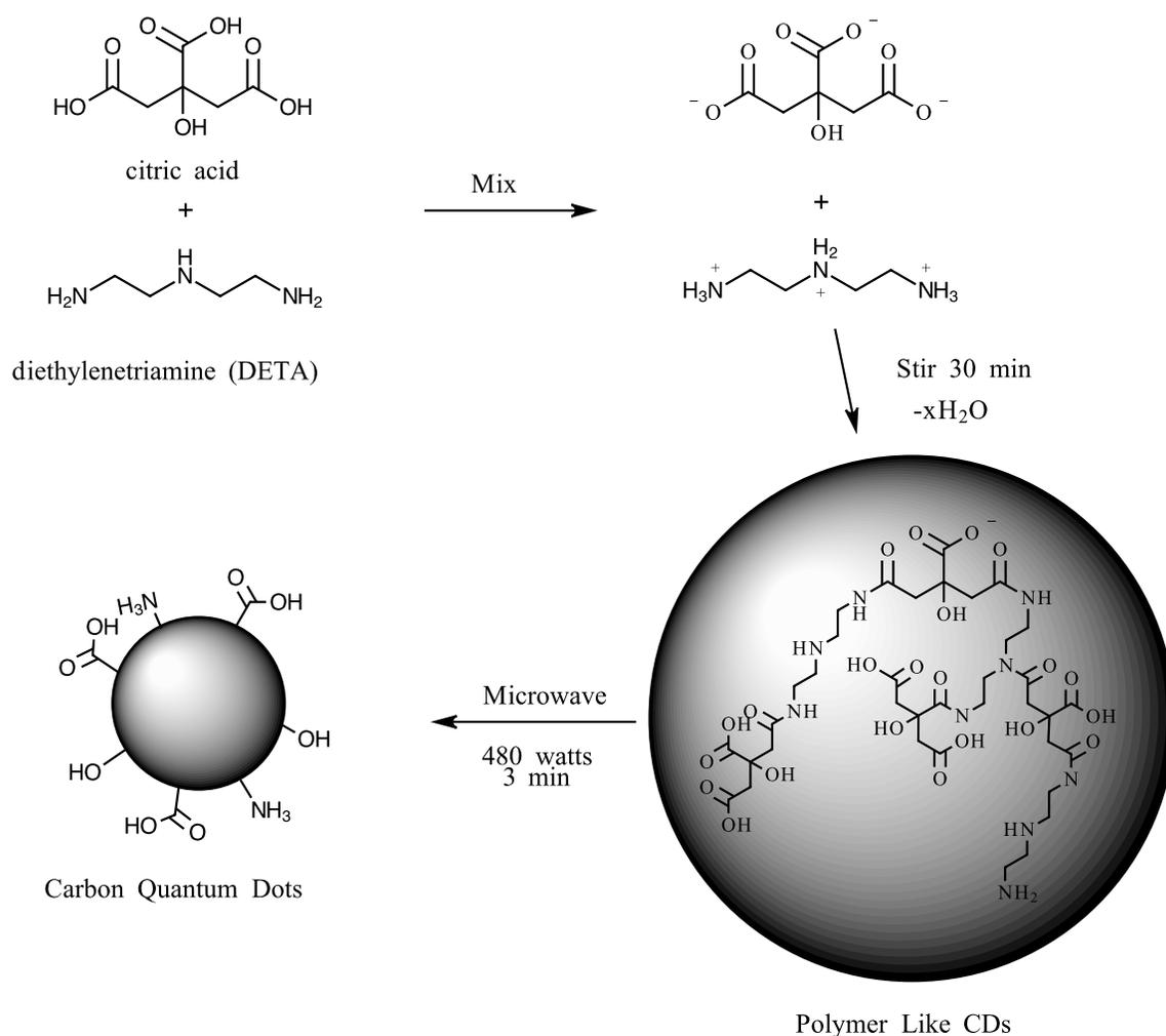
Figure 1. Microwave Synthesis of Carbon Quantum Dots.
