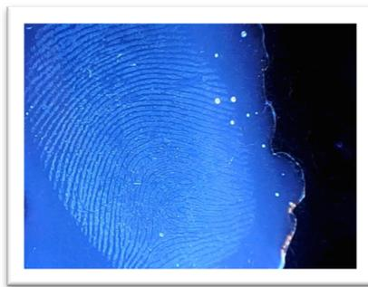
Figure 4. Sample of PVA/CD Latent Fingerprint under 395 nm UV Light.
