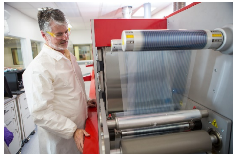
Figure 3 Devin McKenzie demonstrates flexible solar cell printer.
