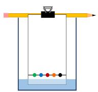
bottom in the water. It is important that the water level is below the line you drew. The final setup should resemble the included diagram.
