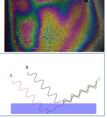
Research Connection: In nanotechnology often properties emerge that are not present in bulk materials. In this case the layer is approximately 1 micron in thickness. This interference of light is used to measure thickness in an instrument known as an ellipsometer. Thin films are using for ant-reflective coatings on windows and solar panels which can control the light of a given wavelength that is reflected or absorbed.
