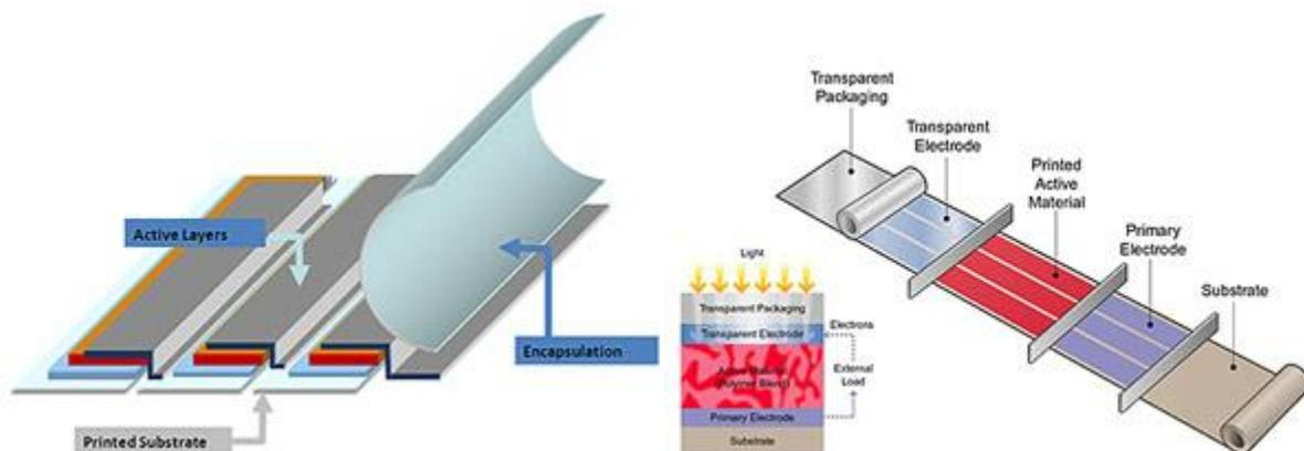
Organic photovoltaics are comprised of several thin layers of carbon-based molecules. The active material is an organic polymer that absorbs light, separates charges, and causes current to flow. The active layer is sandwiched between a transparent conductor, metallic conductors and airtight packaging material. They have a low efficiency of 3-5%. Improving this is an area of active research.
