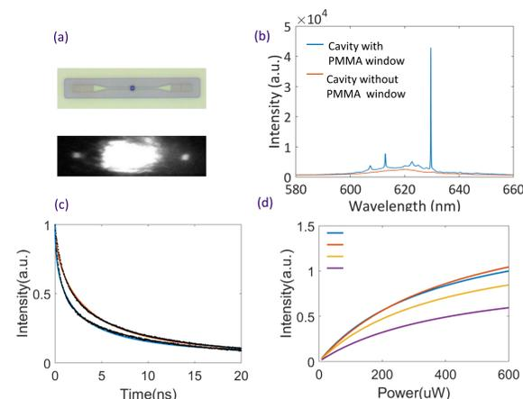
Figure (a) SEM and microscope image of deterministically positioned colloidal CdSe/CdS quantum dots on silicon nitride nanobeam cavity. (b) Spectrum of the cavity-coupled QD emission. (c) Purcell enhancement of QD's emission. (d) Cavity-coupled PL emission intensity normalized by the cavity mode area in different window sizes.
