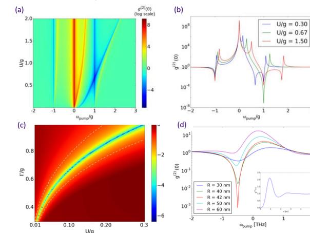
(a)  $g^{(2)}(0)$  versus pump laser frequency relative to the exciton resonance for different values of  $U$  (b) Horizontal cross section of different  $U/g$  (c) Minimum  $g^{(2)}(0)$  for different  $r$  and  $U$ . A 2D plot of the minimum value of the  $g^{(2)}(0)$  that appears at negative pump frequency (d)  $g^{(2)}(0)$  vs pump laser frequency for different Radiuses of the patterned 2D material island
