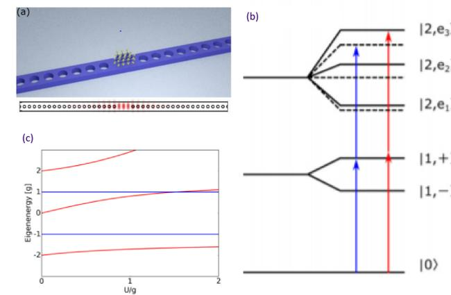
(a) Schematics of the patterned 2D TMDC monolayer on silicon nitride nanobeam cavity (b) Energy level diagram of the dressed states. (c) Eigenenergies as a function of the nonlinearity  $U$ , normalized by the exciton-photon coupling strength  $g$
