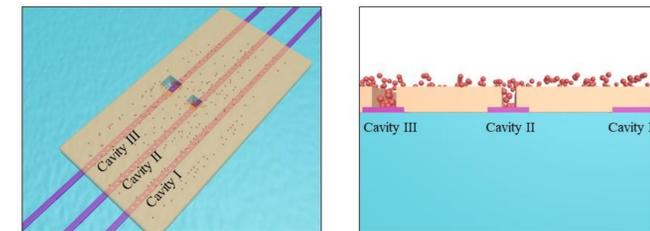
Schematic of deterministically positioned solution-processed quantum dots on silicon nitride nanobeam cavities.
