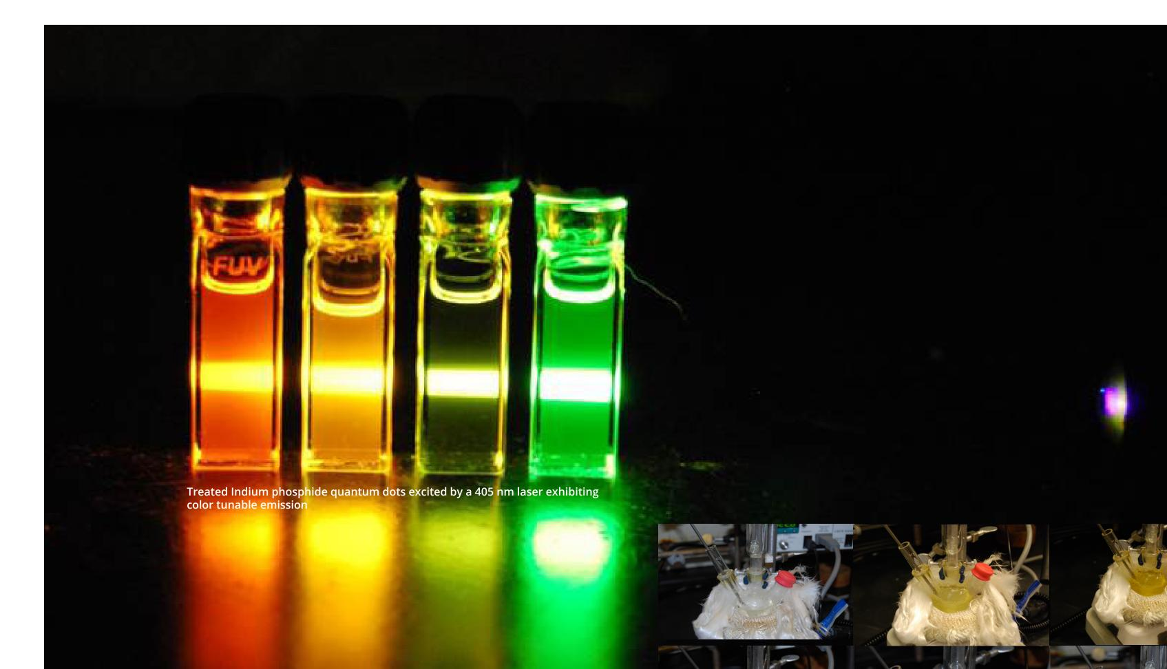
As a quantum dot reaction progresses, the particles grow larger and are able to absorb more visible light due to the quantum confimement effect.
